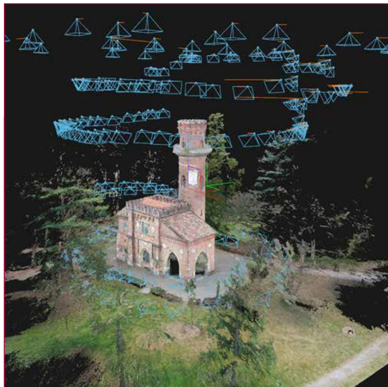
Fig. 2 - Aerophotogrammetric data processed in Cube-3d.
