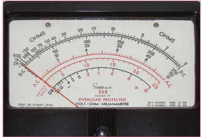
Fig. 9 - The old analog multimeter with the concentric scales and the common pointer. The three inside scales (black, red and red arcs) have equal subdivisions of Volts/milliamperes (DC-AC). Note that the concentric scales of Ohms and Decibels do not have equal subdivisions.
