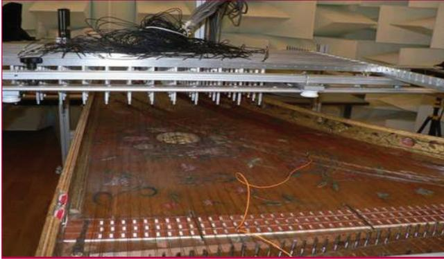
**Fig. 6 - Acoustic holograph of the J. Couchet harpsichord**
