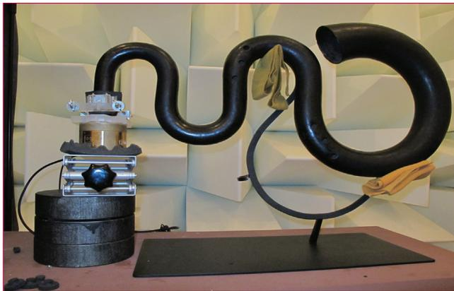
**Fig. 4 - Acoustic impedance experimental setup**
