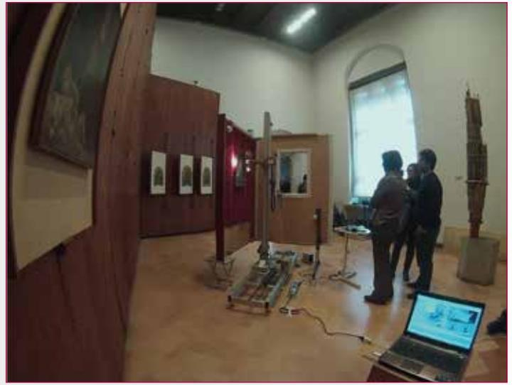
Fig. 2 - Palazzo Abatellis, Sala di Antonello, in situ investigations using INTRAVEDO equipment, an ultra-high-resolution IR and XRF scanner.
