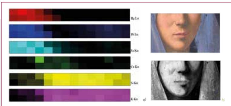
Fig. 5 - Antonello da Messina, *Annunciata*: a) mercury, lead, iron, copper, silicon and potassium line maps. The iron is totally absent in the area of the veil that in the past was affected by a dark layer of ochre or earth to define the shadow.
