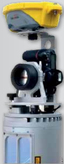
Fig. 1 - Example of integration among three sensors: laser scanner, photo camera and GNSS unit.
