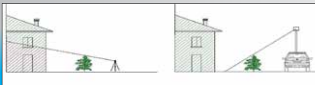
Fig. 2 - Zones of undercut due to the presence of obstacles.
