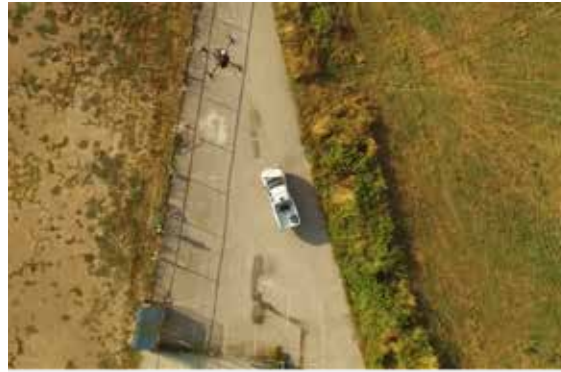
Fig. 10 - Tethered drone used on mobile pick-up
