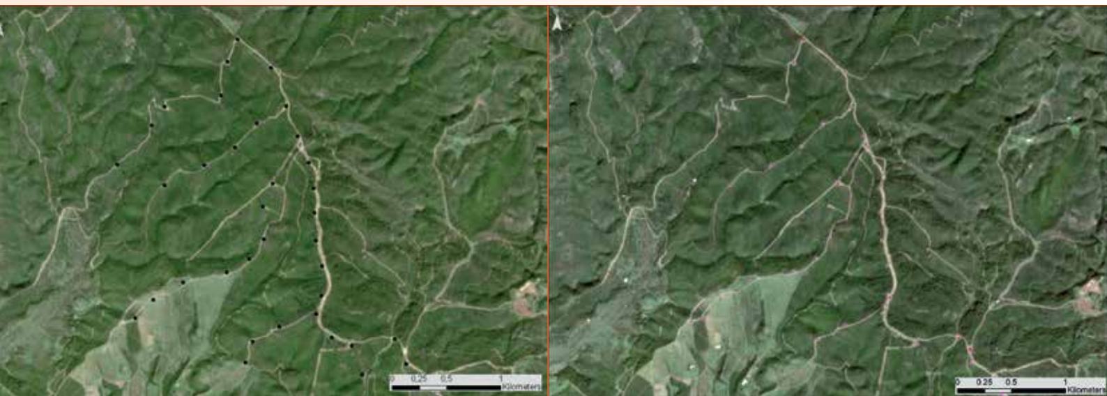
Fig. 2 - a) actual positions (black points) of the wind turbines of a wind field and b) detection results in an example location of the study area (Villaurbana – OR).
