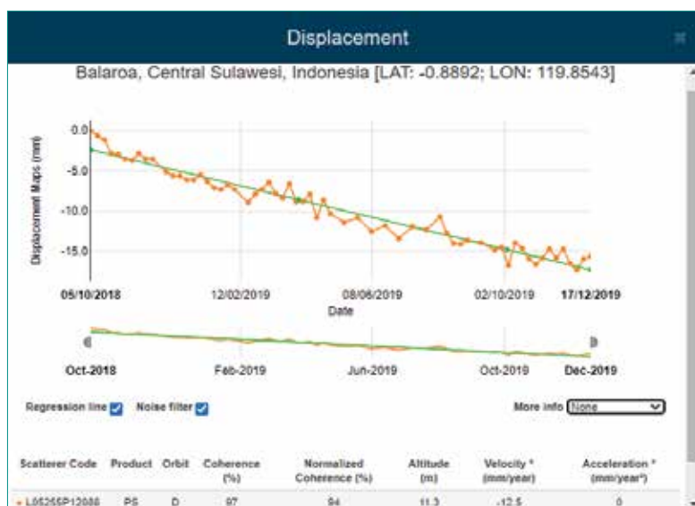
Fig. 4 - Example of one PS displacement (mm) over time computed through the PSI over Palu area after the earthquake. In this figure it is possible to see all the geo-analytics and filtering tools for the exploitation of the ground motion map.
