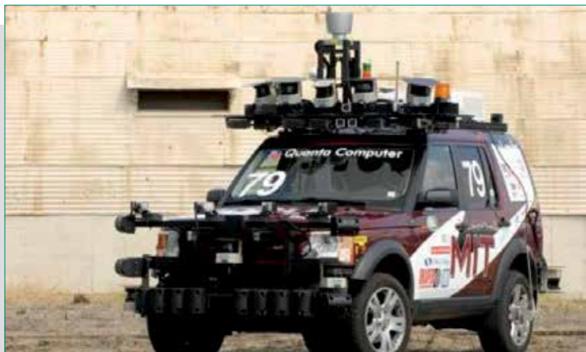
Fig. 1 - Land Rover's fully autonomous LR3 created by Team MIT for the DARPA Urban Challenge (2007).
