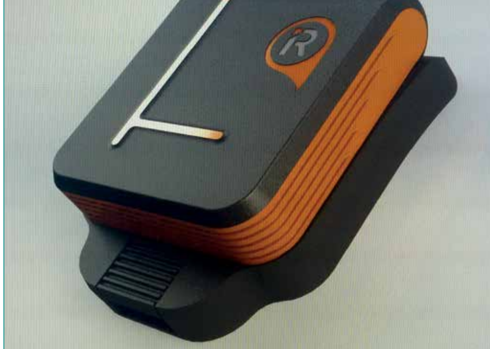
Fig. 5 - 3D model of the first responder's wearable for improved positioning and environmental sensing.
