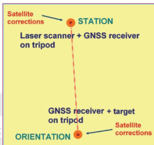
Fig. 2 - Direct geo-referencing for scanning survey.
