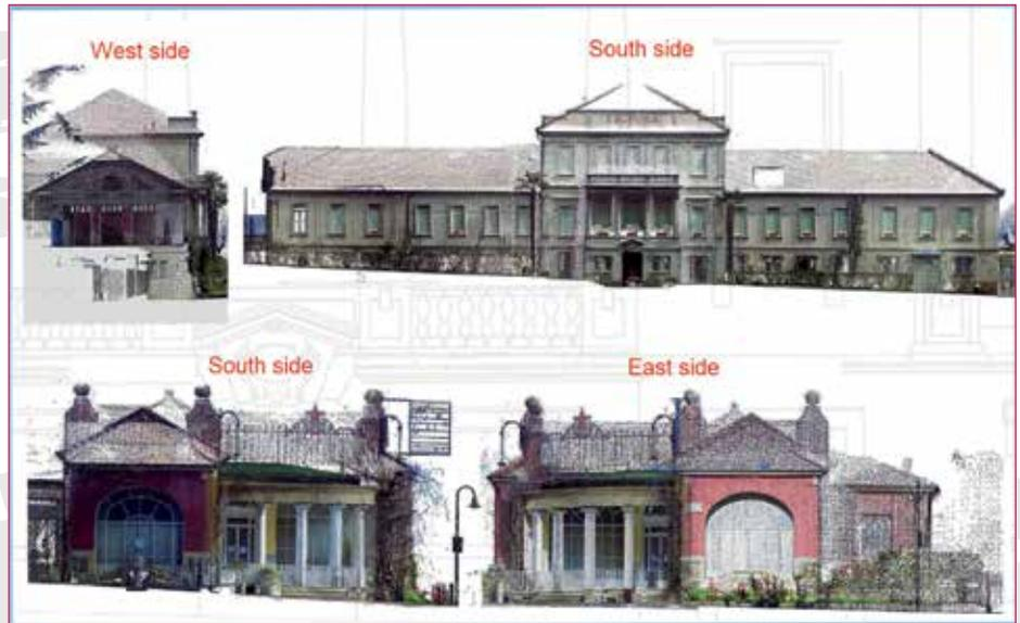
Fig. 6 - Orthographic elevations of the Spa-buildings, extracted from the point model.
